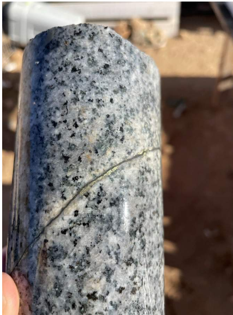
Cpy-py-mag mineralisation in fracture vein, SLD005.
