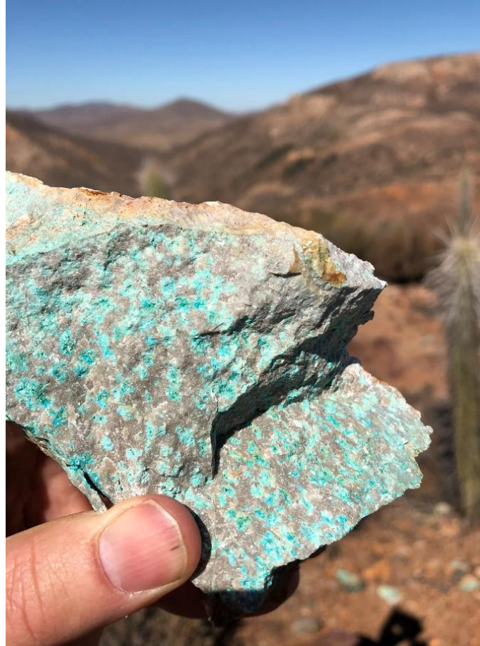
Disseminated high grade copper hosted in advanced argillic high sulphidation alteration
