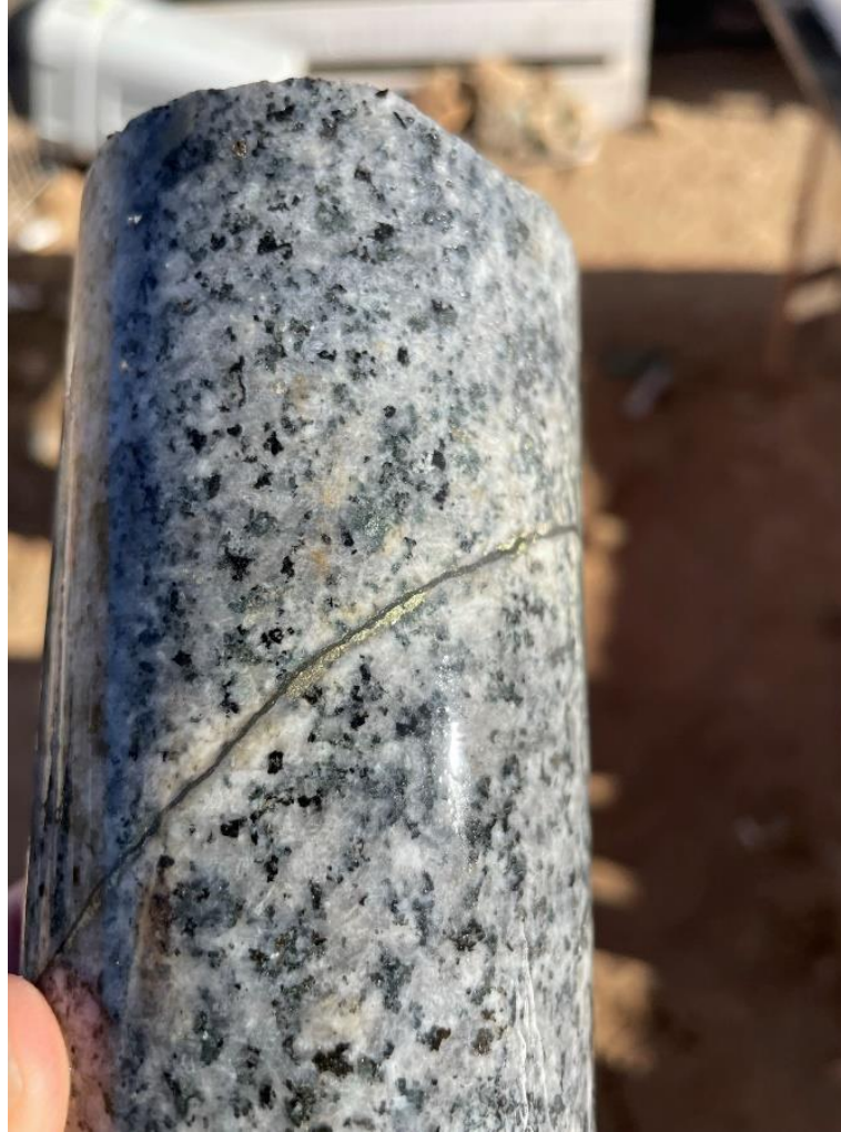
Cpy-py-mag mineralisation in fracture vein, SLD005.
