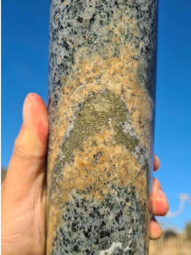
Coarse cpy vein with Kspar halo, SLD008 Central prospect.
