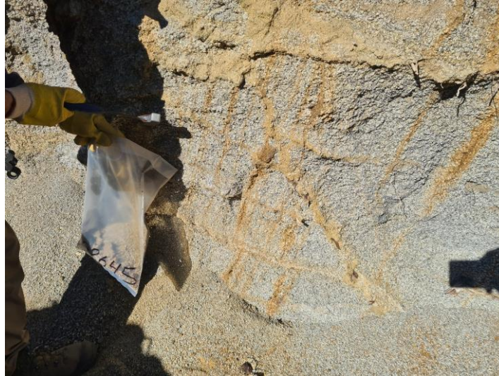
Sampling trench CWT002, Chinchillon zone highlighting oxidized fracture-vein swarms
