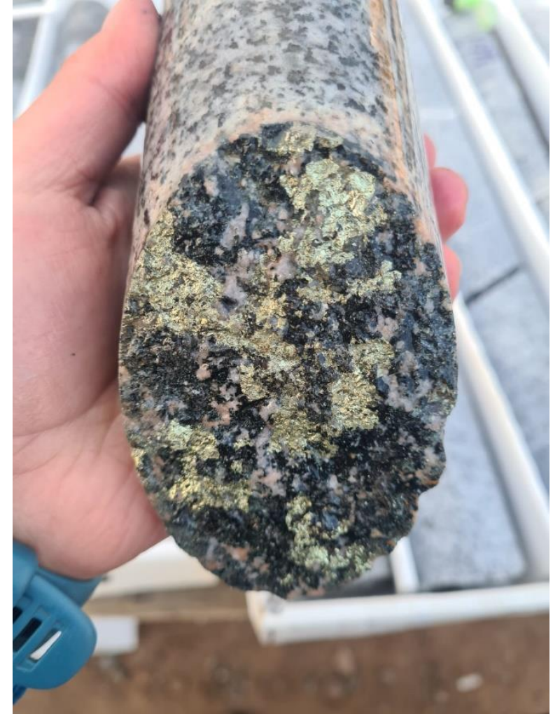
Cpy-act mineralisation on fracture-vein, SLD008.
